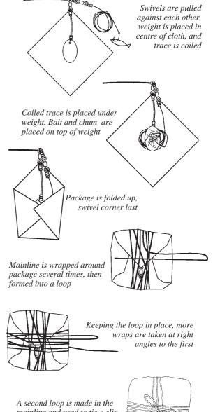
mainline and used to tie a slip knot with the first loop
