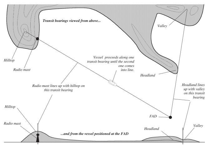
The fisherman should always be able to approach the FAD by first lining up one of the transits, and then following the transit line until the landmarks of the second transit are also in alignment.
