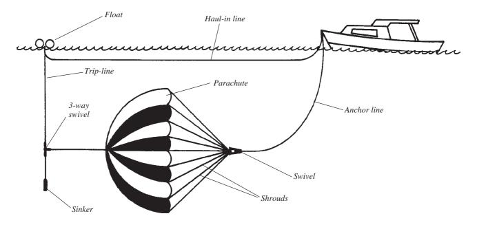
The anchor line is a length of strong rope, 20–30 m long, of the same diameter that would be used by the vessel if it were using a normal ground anchor. One end is connected to the shrouds of the sea anchor, the other to the boat.
