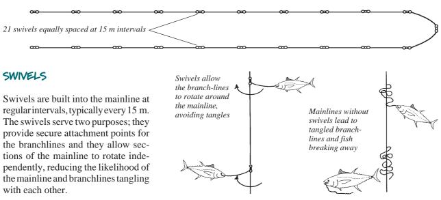
Heavy duty swivels made of brass or stainless steel should be used. Brass barrel swivels function almost as well as stainless steel ball-bearing swivels and are available at a fraction of the cost.
