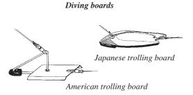
The trolling depth of the board depends on the size of the board, the speed of the boat, and the amount of line you pay out. Once the board reaches its maximum depth, it will (usually) stay there and remain steady provided that it is properly balanced. When a fish hooks up on the lure, the added weight on the line alters the board's angle and causes it to trip and rise to the surface, dragging the fish along with it.
