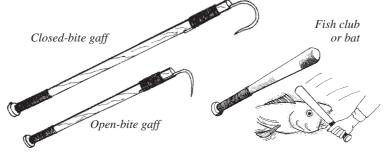
A couple of gaffs and a fish club or bat are essential equipment when fishing around a FAD. A large fish should be gaffed through the head and then stunned with a fish club as soon as it has been brought on board. This not only stops the fish from causing injuries, but also prevents damage to the fish flesh which could reduce its value.
