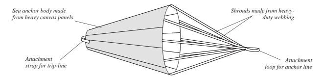
An important feature of a sea anchor is a vent at the top of the parachute which allows water to flow through. This is an essential feature which allows the sea anchor to fill properly when deployed and to empty when retrieved. It also helps prevent the anchor from tearing when the pull is very strong. On commercial sea anchors, a webbing strap is stitched across the vent and this serves as the attachment point for the trip line (see below).
