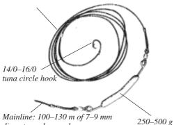
diameter polypropylene rope lead-filled copper tube with 30-degree bend (to prevent rolling)
