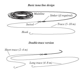
The line would normally be weighted with a sinker heavy enough to carry the bait down to the desired depth under the prevailing wind, current and fishing conditions. In a strong current a sinker of 1 kg or more may be needed, while in a light current a relatively small sinker of 100–200 g could be used. If drifting in a light current it may be possible to fish with no sinker at all, especially if a leaded swivel is used in the line.
