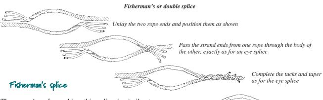
The procedure for making this splice is similar to making two eye splices. However instead of splicing the end of a rope back into itself, two ropes are used, with the end of each one being spliced into the standing part of the other.
