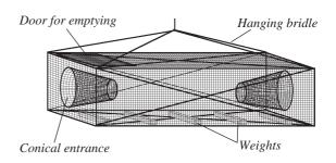
The traps generally worked well when suspended from FADs known to regularly aggregate baitfishes. A typical daily catch in one location was 30–60 pieces of bigeye scad or mackerel scad, with the best catch being 140 pieces.
