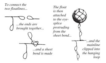
The result is two lines fishing while tied off in sequence from the boat. Additional lines can be connected to the end of the string, which can either be left tied to the vessel or can be detached once a sufficient number of lines have been strung together.
