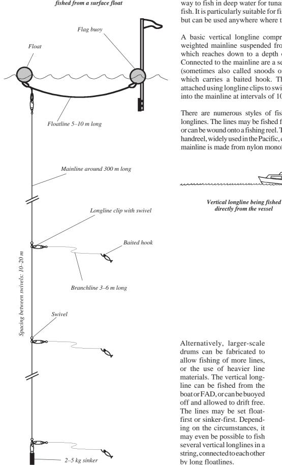
Vertical longlining is a simple and relatively cheap way to fish in deep water for tunas and other oceanic fish. It is particularly suitable for fishing around FADs but can be used anywhere where tunas are found.
