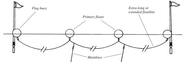
Normally strings of lines are set using the sinker-first method. Technically it should also be possible to set strings using the float-first method, but this would require motoring the boat back to the float of each line after it had been set in order to connect the next line to it. Since this rather defeats the object of the float-first method, whose main advantage is speed, this technique does not actually appear to have been used.
